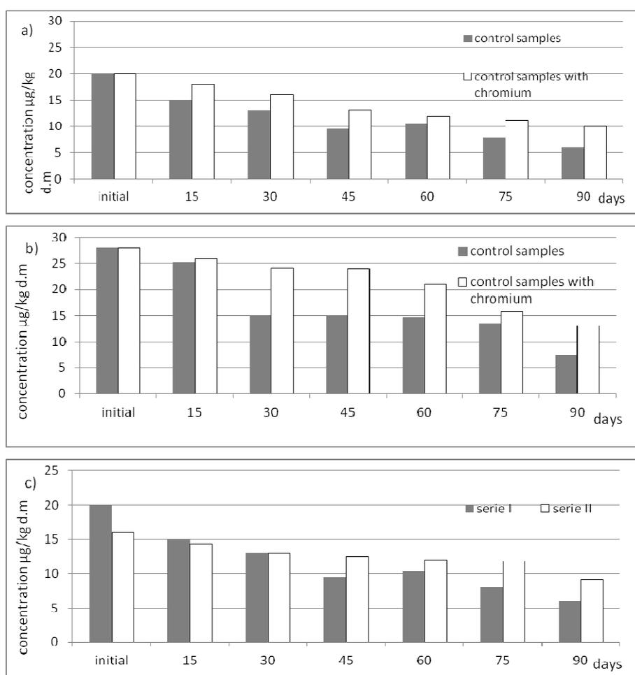
Fig. 4. The changes of fluorene concentration in samples: a) serie I, b) serie II, c) abiotic samples
