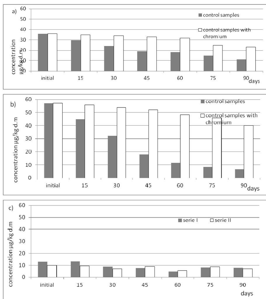
**Fig. 6.** The changes in the concentration of anthracene in sewage sludge: a) serie I, b) serie II, c) abiotic samples
